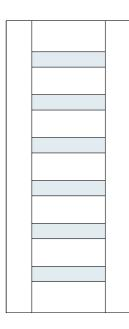
Modified TM6100 in MDF with One Step (OS) sash and Paper Cut resin inserts
