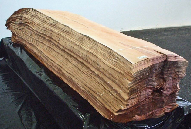
The sheets are then bundled in sequence for sale. TruStile purchases as many sequenced bundles as possible within our grading requirements.
