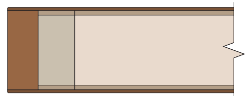
1-3/4" Flush Wood Door Cross Section
